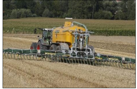
Applying fertiliser by a trailing hose.
